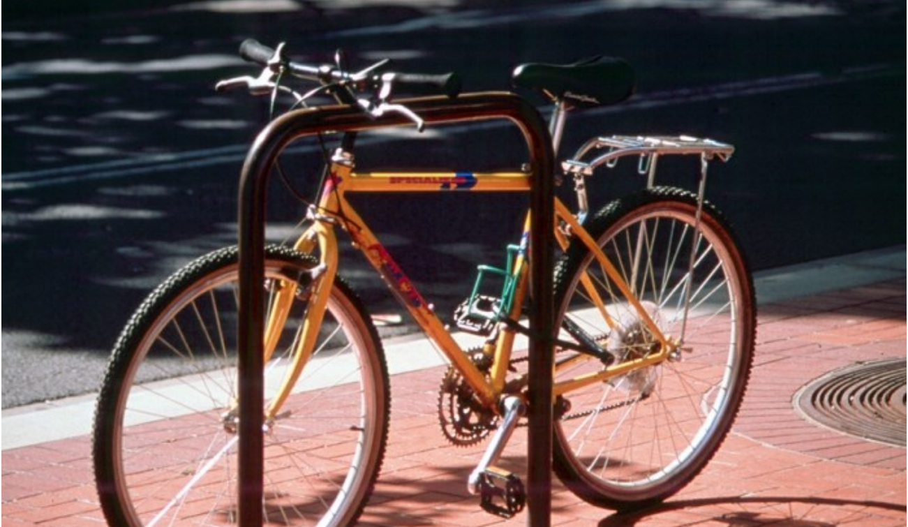
Bicycle racks should support the bicycle at both the tire and the frame.
