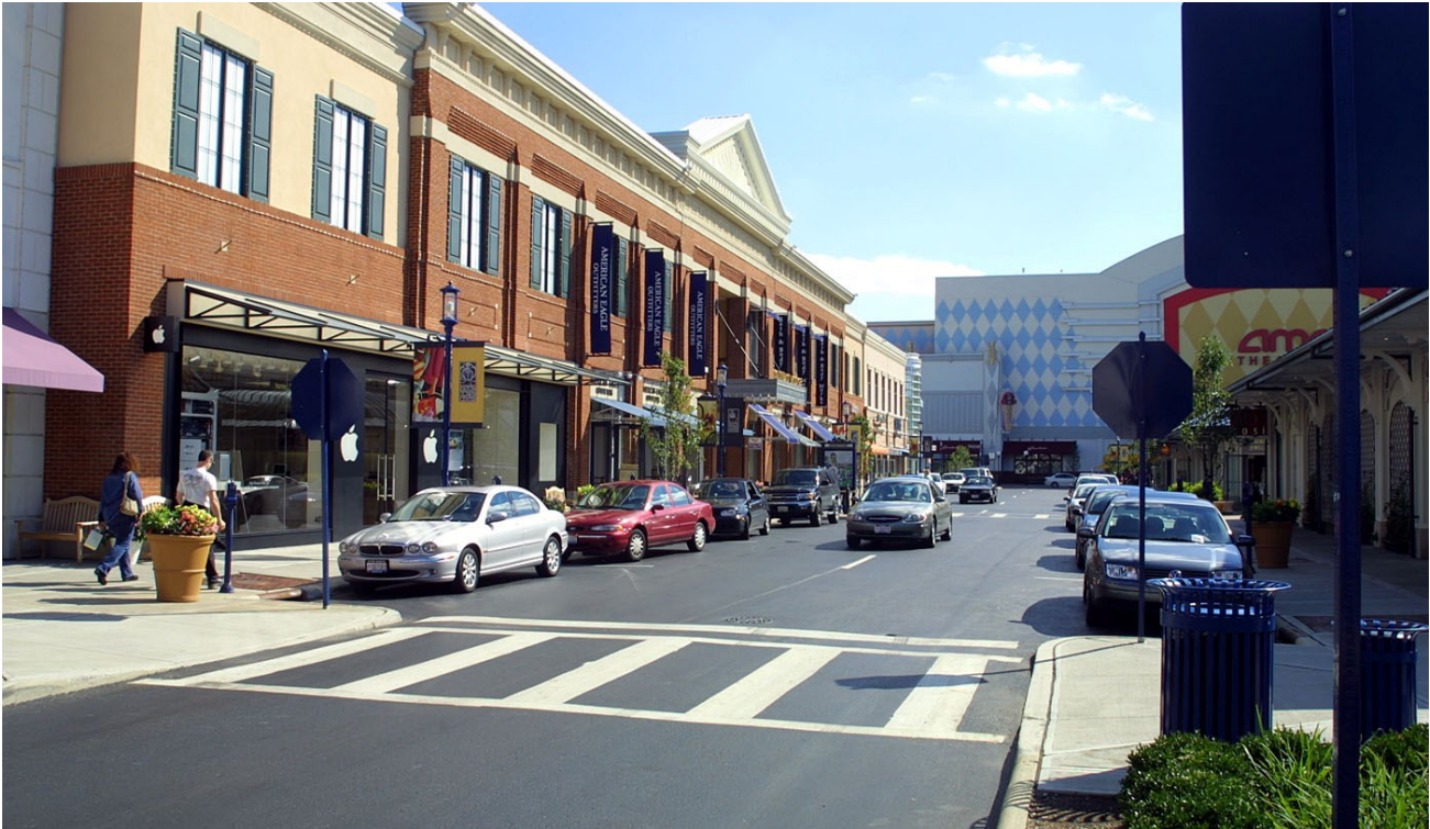
Ladder style crosswalk with bump-out to reduce the distance pedestrians have to cross
