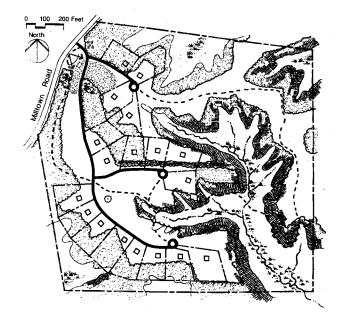
Figure 15 Step Four Drawing in the Lot Lines
