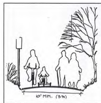
Figure 3 Recommended widths for bicycle paths (AASHTO, 24)
