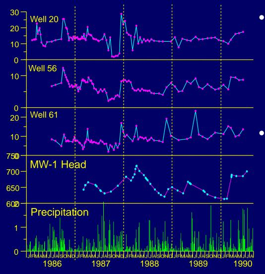
NO<sub>3</sub>-N values from three domestic wells completed in the Silurian dolomite (miles apart)
